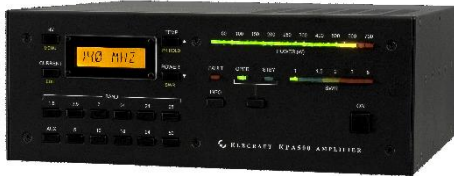
KPA500 Solid State, 500W, Automatic Band-Switching Amplifier
